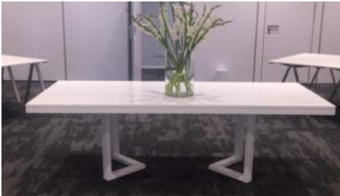
BRIEF: Manufacture 16 x Banquet tables, as per design detail supplied. Removable steel legs, powder coated white; 32 mm supra-wood top with high gloss K2 finish. Size: W1000 x L2400 x H750. Completed tables above in situ
